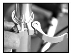
If the quick release feels too loose, use the adjustment finger nut to increase the tension (see **photo left**). Properly adjusted, the quick release requires a firm hand to close. The steering tube should never be able to telescope down when you put your body weight on the handlebars. If so, tighten again.
