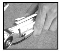
An easy way to free up the pins so that they open easily is to give the vehicle a little shake while simultaneously squeezing the levers. When the vehicle is in the folded position, leave it flat on the ground when releasing the levers.
