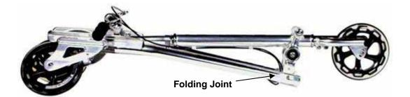
At the front of each leg you will find a folding joint with a finger lever on either side. Squeezing the levers simultaneously unlocks the mechanism (photo right). Once released, simply swing each leg into its fully open position. Each lever will lock in the fully open or fully closed leg position. Please note that these mechanisms can feel sticky, but the culprit is usually pressure in one direction or the other on the locking pins inside the mechanism.
